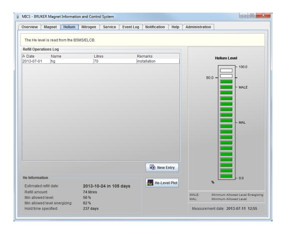
After helium refill, the refill information needs to be entered on the *Helium* tab. Press the button *New Entry* to access the editor and to enter the helium refill information.
