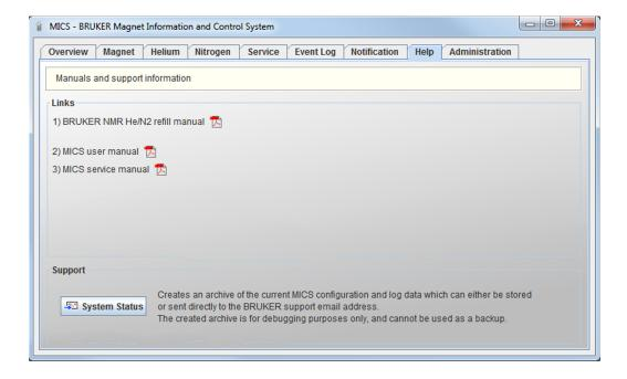
The Support section provides a tool to create a zip archive of the current MICS configuration and logfiles. Press the button System Status to create an archive containing the following data:
