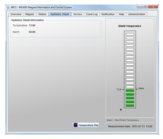
MICS displays the radiation shield temperature in Kelvin. The shield temperature can also be displayed in a 2D plot, using the button *Temperature Plot*.
