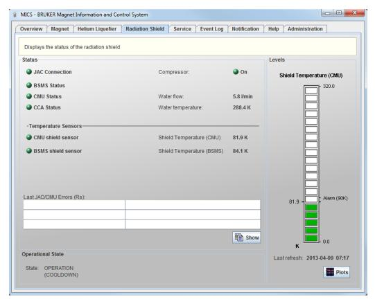
MICS displays the radiation shield temperature in Kelvin as a temperature gauge. The shield temperature and other parameters can also be displayed in a 2D plot, using the button *Plots*.
