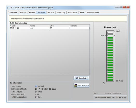
Each time after refilling nitrogen, it is important to enter this information in MICS. Start MICS and select the *Nitrogen* tab. Update the refill table by pressing *New Entry*. This is particularly important if the magnet system is not equipped with a nitrogen level measurement device (see information below).
