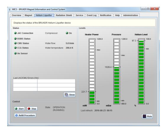
The *He Liquefier* tab displays all relevant information regarding the He liquefaction unit. Heater power, He pressure, He level and other parameters can also be displayed in a 2D plot, using the button *Plots*.
