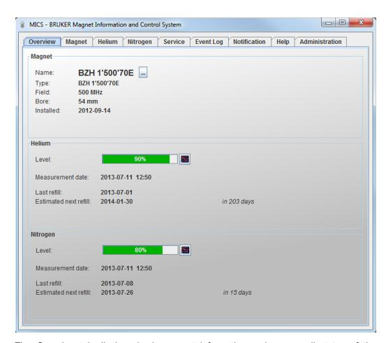
The *Overview* tab displays basic magnet information and an overall status of the cryogenic agents of the magnet system. It is possible to change the magnet name according to individual needs. This name will be used in email notifications and other MICS messages.
